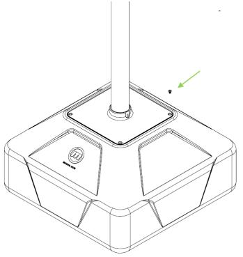
Using Thread lock and the 4 Flathead Screws, secure the cap to the base.
