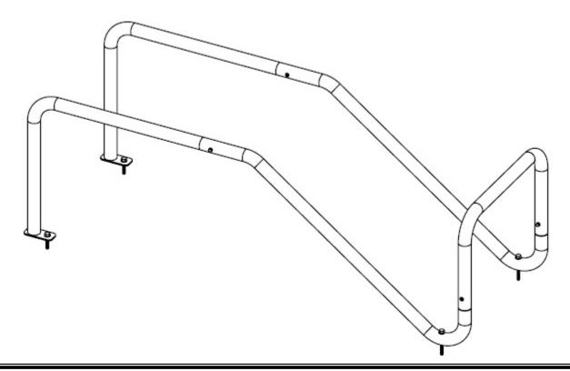
**IMPORTANT:** Assemble on a flat, level surface. All cart corrals should be inspected on a regular basis for damage. McCue recommends a minimum of two inspections per year in the spring and fall. Any damaged pieces, including ground frames and lane dividers which are not flat and flush with the ground, should be replaced with McCue replacement parts.
