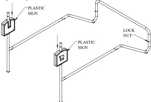
Attach crossbar with unsecured signs to the front of the unit Lift crossbar onto the front uprights and align holes. Make sure uprights are standing vertical.
