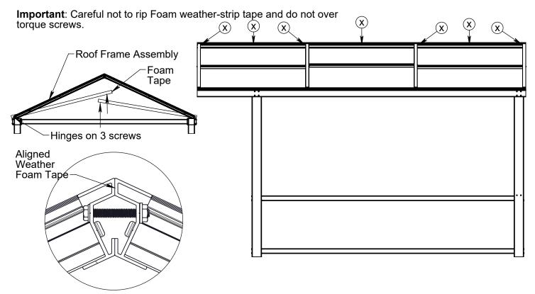
Step 6B: Secure Roof Frame Assemblies to Toprails.
