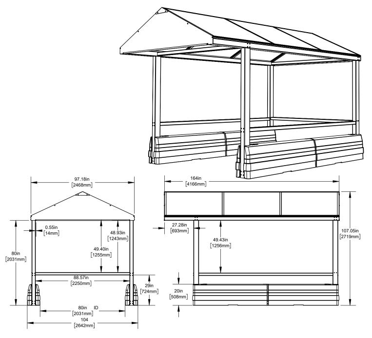
IMPORTANT: Assemble on a flat, level surface. All cart corrals should be inspected on a regular basis for damage. McCue recommends a minimum of two inspections per year in the spring and fall. Any damaged pieces should be replaced with McCue replacement parts.
