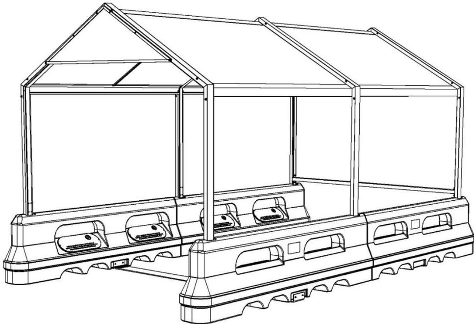
**IMPORTANT:** Assemble on a flat, level surface. All cart corrals should be inspected on a regular basis for damage. McCue recommends a minimum of two inspections per year in the spring and fall. Any damaged pieces, including ground frames and lane dividers which are not flat and flush with the ground, should be replaced with McCue replacement parts.
