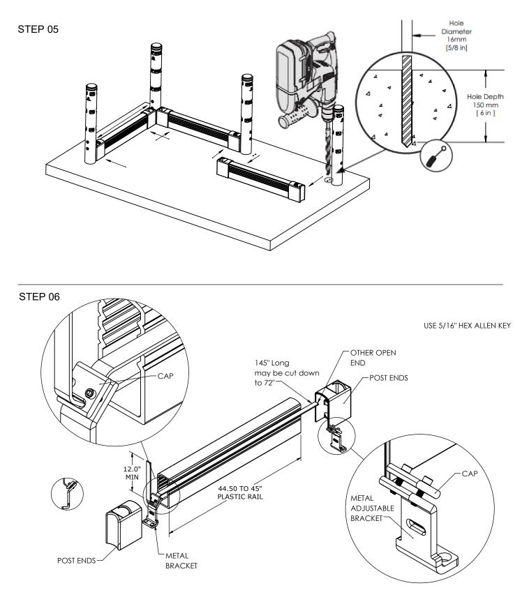
PULL THRU PLASTIC STRAP 12" MINIMUM PAST CAP AND SECURE CAP TO METAL ADJUSTTABLE BRACKET WITH (2) 3/8-16 X 1.50" SOCKET HEAD CAP SCREWS USING A 5/16" ALLEN KEY. ALTERNATE BETWEEN SCREWS FOR AN ACCURATE TIGHT HOLD.
