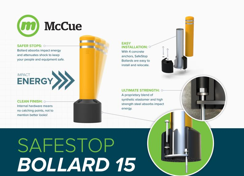
Meet SafeStop Bollard 15, our impact-absorbing bollard engineered to stop heavy equipment. SafeStop Bollard 15 safely absorbs and withstands impacts up to 15,000 J, keeping your people safe and your facility damage-free.
