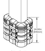
Column Guard Minimum Column size [200mmx200mm]
