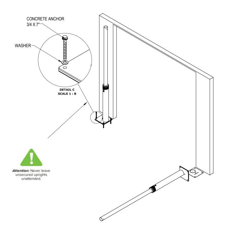
7 STAND UPRIGHT OVER RUBBER TEMPLATE, ALIGN ALL THE HOLES AND SECURE POST TO CONCRETE WITH (5) 3/4"X 7.0" ANCHORS AND (5) FLAT WASHERS UNTIL FLUSH WITH TOP OF PLATE. MAKE SURE ALL FASTERNS ARE TIGHT.
