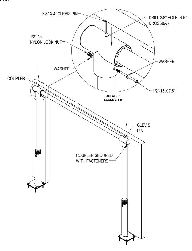
(9) GOAL POST IS COMPLETE WHEN ALL FASTENERS ARE SECURED AND CLEVIS PINS ARE INSTALLED.
