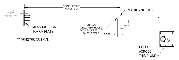
4 CUT CROSSBAR IF NEEDED (YES OR NO) IF YES, MEASURE BETWEEN THE RUBBER TEMPLATE LINES TO GET YOUR WIDTH. DOUBLE CHECK YOUR WIDTH PRIOR TO CUTTING. USE A METAL CUTTING BLADE TO CUT CROSSBAR. THRU. CLEAN CUT EDGES IF NEEDED WITH A METAL FILE.
