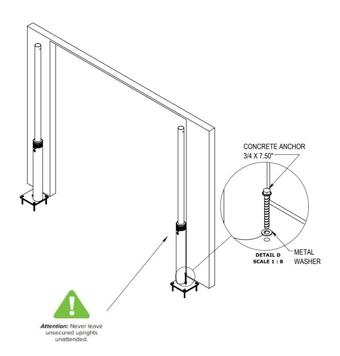
(8) USING A SCISSOR LIFT, SLIDE COUPLERS ON THE CROSSBAR ENDS, AND SLIDE ONTO POSTS.
